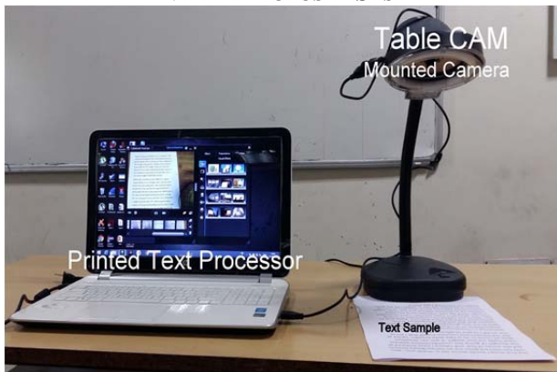
Figure 2. First prototype of the proposed system consisting of a computer system with OCR and Text-to-speech processor, and a table CAM with camera mounted on the top inside.
